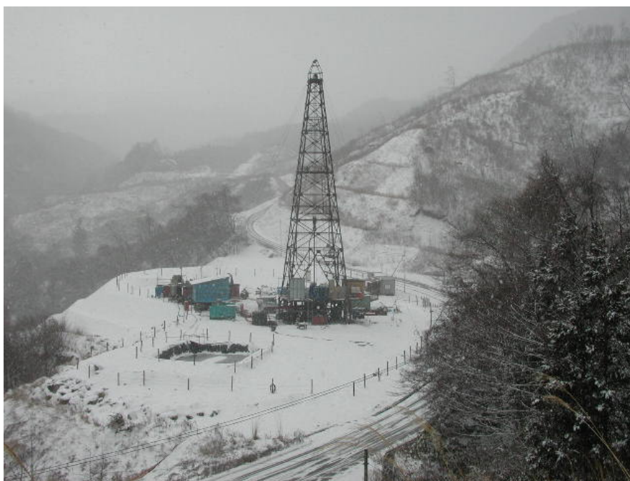
Figure 13.6 Drilling for exploration well in Ten'ei (Middle of Honshu) geothermal field, research activities under Survey Program C-2 started FY2004 (Nov 2004).
