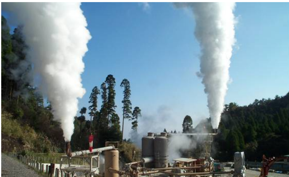
Figure 13.4 Production test for exploration well in Kirishimaeboshi-dake (South side of Kyushu) geothermal field, research activities under Survey Program C-1 conducted by NEDO, started from FY2001 to FY2004. Flow rate: Steam 40t/h, water 120t/h (Nov. 2004).
